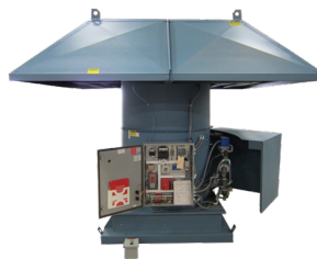
Vertical and Horizontal Econo Unit for lower cost alternative to make-up air problems. Heating capacities from 950,000 to 2,900,000 BTU. Airflow up to 23,500 CFM at static pressure of 1/4" Series 78H, 78V
