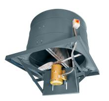
**The Series 61** meets the need for an economical, yet efficient upblast roof ventilator. The unit combines the Hartzell panel fan concept with a windband and butterfly damper. Dampers open automatically when the fan goes on and close weather tight when the fan is shut down. When the unit is in operation, the force of the discharge air effectively prevents the entry of rain or snow.
