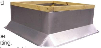
All prefabricated curbs can be furnished for slope or peak bases. Prefabricated curbs are designed to support the weight of the fans cataloged herein and attachments not exceeding over 100 additional pounds in a 40 mph wind. Nonstandard curb construction is available.
