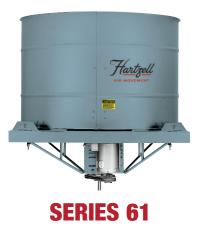
Meets the need for an economical, yet efficient upblast roof ventilator. The unit combines the Hartzell panel fan concept with a windband and butterfly damper. Dampers open automatically when the fan goes on and close weather tight when the fan is shut down. When the unit is in operation, the force of the discharge air effectively prevents the entry of rain or snow.
