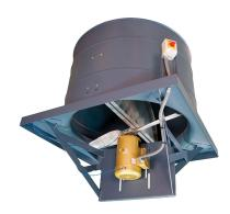
The Series 61 meets the need for an economical, yet efficient upblast roof ventilator. The unit combines the Hartzell panel fan concept with a windband and butterfly damper. Dampers open automatically when the fan goes on and close weather tight when the fan is shut down. When the unit is in operation, the force of the discharge air effectively prevents the entry of rain or snow.
