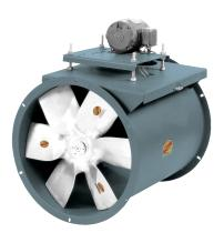
The Series 46 fan features a six-blade, cast aluminum, airfoil propeller mounted with split-taperlock brushing and a safety retainer plate for easy installation and removal. The one-piece housing is constructed of heavy-gauge, hot-rolled steel with a continuously welded steel drum and flanges. Series 46 Duct Axial® Fans are also available with an aluminum housing.
