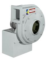
The Series 42 & 43 can handle the low flow and high pressure situations and perfect for wet-well ventilation. Just like the Series 41 the blowers wheels are a solid one piece molded fiberglass construction and made of Derakane 510-A.
